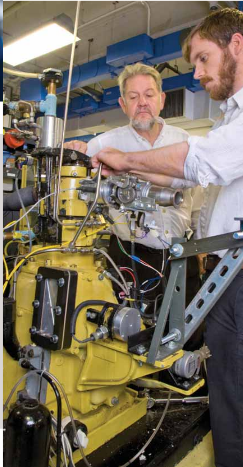
Professor Robert Dibble (left) and post-doc Hunter Mack install the pressure transducer in the head of the combustion chamber on a single-cylinder Waukesha CFR engine, an industry prototype for researching internal combustion engines.
