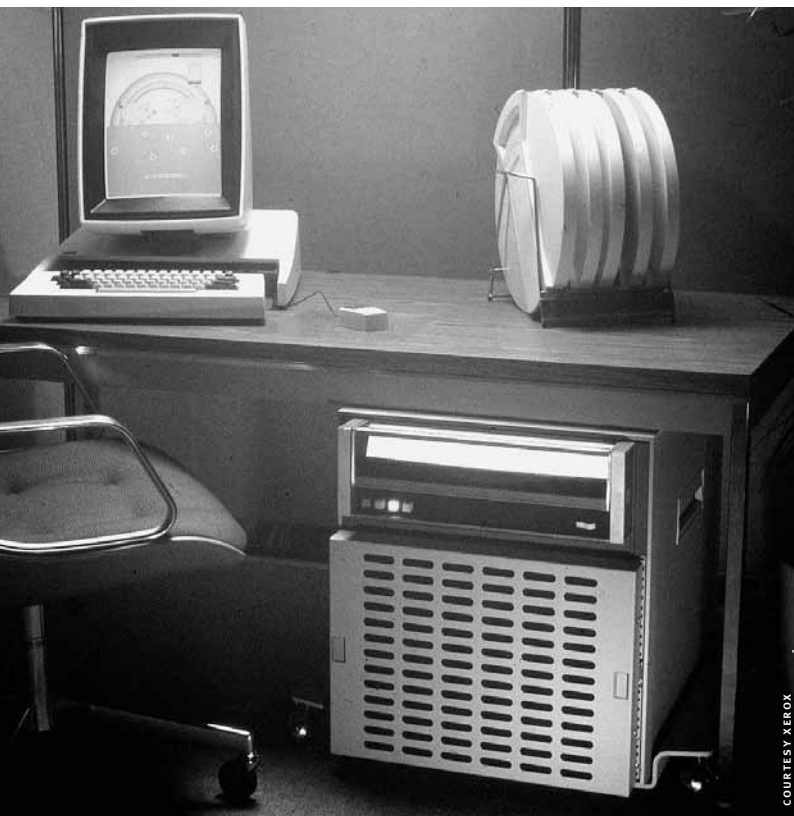
The Xerox Alto—built by Project Genie alumni Butler Lampson, Peter Deutsch, Chuck Thacker and colleagues at Xerox PARC in the early 1970s—is considered by many to be the first personal computer. The air-conditioner-sized unit under the desk contains the computer's printed circuit boards.
