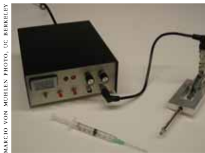
The MicroJet won't entirely replace the hypodermic needle (foreground), but its comparative precision could facilitate its use in microsurgery and in delivering arthritis drugs into joint areas too shallow for a needle to penetrate.
