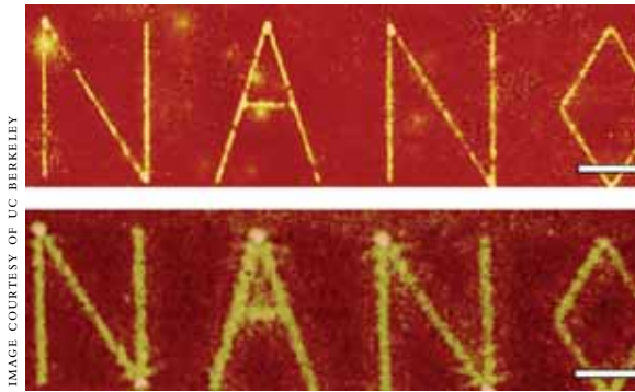
The word NANO, recorded onto an organic polymer, appears sharper in the image created with the silver superlens (top) than that created with a conventional lens (bottom). The scale bar in both images represents 2 micrometers.
