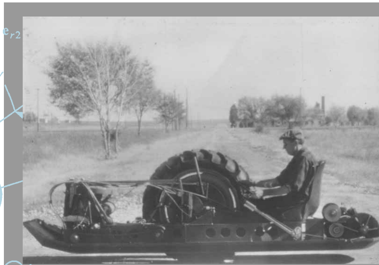
The one-wheeled vehicle, patented by Charles F. Taylor in 1964, used gyroscopes for steering and stability—all before computers were there to assist. Taylor is seen here in 1965, driving the prototype of his vehicle near Golden, Colorado. Go to www.me.berkeley.edu/one_wheel_vehicle/ to download the movie of Taylor and his vehicle.
