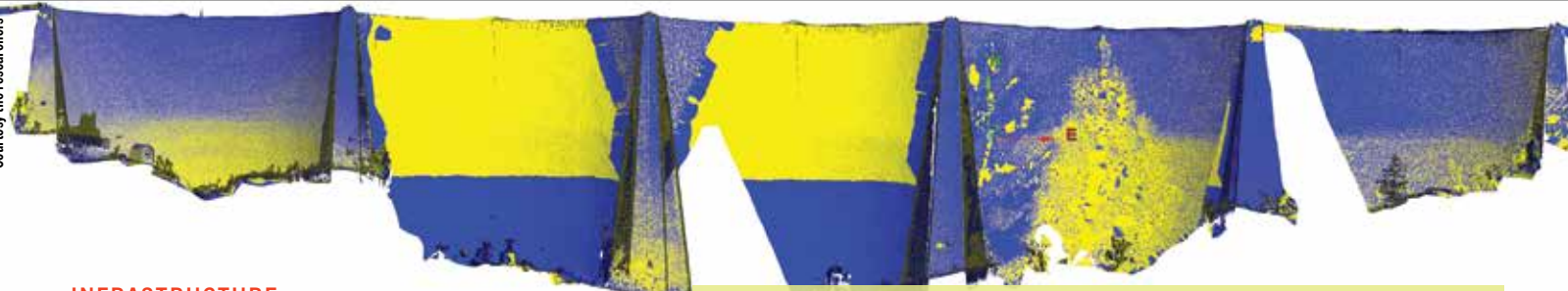
A frontal view of Hume Lake Dam after comparing scans from before and after drainage. The blue color shows where the dam moved toward the reservoir, and the yellow color shows where it moved downstream.
